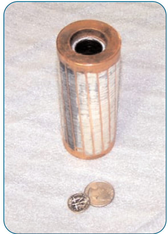
Figure 1. This rotor illustrates the value of copper when combined with good design: it produces eight horsepower but is no larger than a Wisconsin bratwurst.
