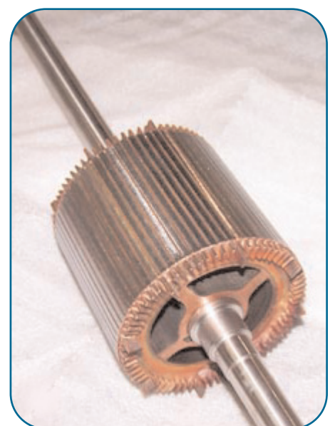
Figure 3. A fabricated 400-Hz copper rotor. Note the large lightening holes in the laminations.
