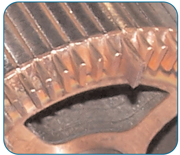
Figure 4. Close-up showing braze joints between conductor bars and the end ring. Fabrication is a tedious and demanding process, but the ability to include cooling fans economically is seen as an advantage.
